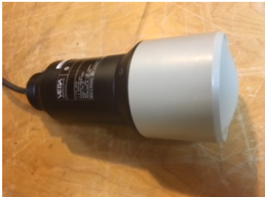
Photograph 1: PSWLS61 with 82mm Encapsulated Plastic Horn Antenna
