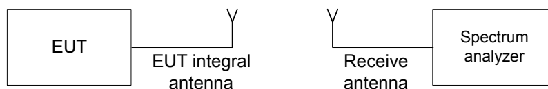
Figure 7.1.1 Setup for transmitter shut down test
