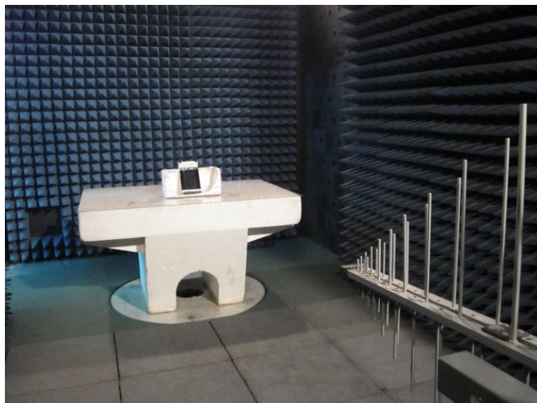
Photograph 8.1.1 Setup for radiated emission measurements
