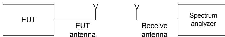
Figure 7.3.1 Occupied bandwidth test setup
