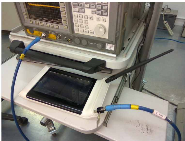
Photograph 8.2.1 Spurious emission test setup
