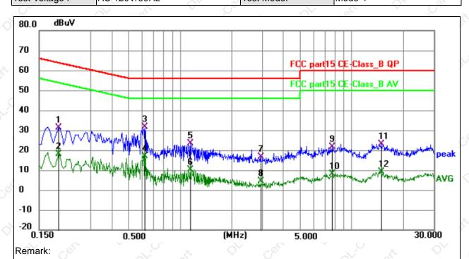
Margin = Limit - Level, Correct Factor = Cable lose + LISN insertion loss, Level= Reading + Correct factor
