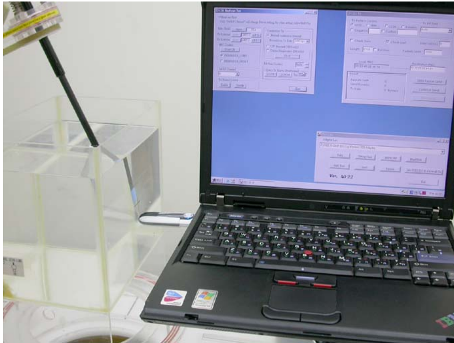
Figure 10: EUT perpendicular to phantom, 0 mm separation
