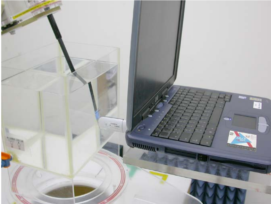
Figure 16: EUT perpendicular to phantom, 0 mm separation
