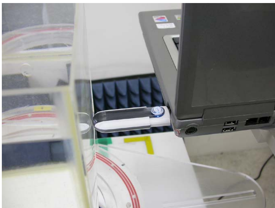
Figure 5: EUT perpendicular to phantom, 0 mm separation- Zoom In
