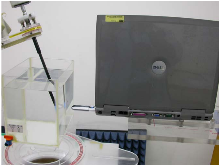
Figure 6: EUT perpendicular to phantom, 15 mm separation
