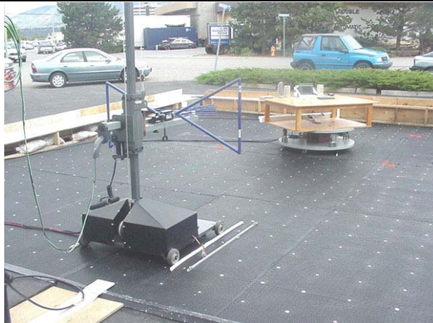
Photograph I.8-4 - 3115 Horn Antenna (2GHz - 10GHz)
