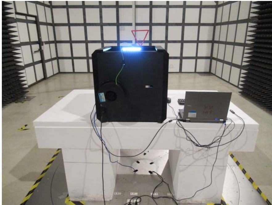
Radiated Disturbances Rear Side (Below 1G)
