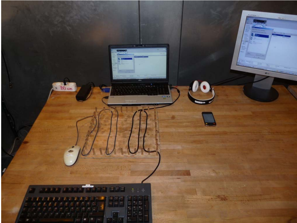
Photo 1: Test setup for conducted measurements (AC Port (power line), computer peripheral setup, EUT supplied by USB-cable from computer, intentional / unintentional radiator §15) Computer supplied by 110v 60Hz AC.
