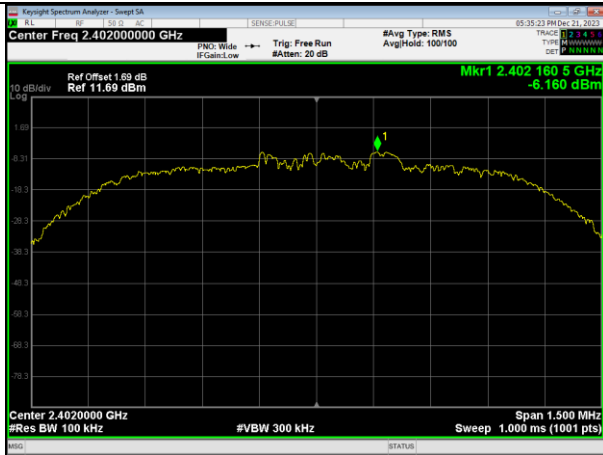
\pi/4 -DQPSK on Channel 39
