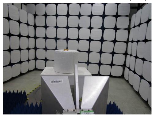
1.2 Field Strength of the Fundamental Signal Test setup
