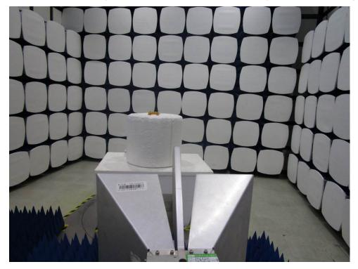
1.3 Radiated Emissions Test Setup
