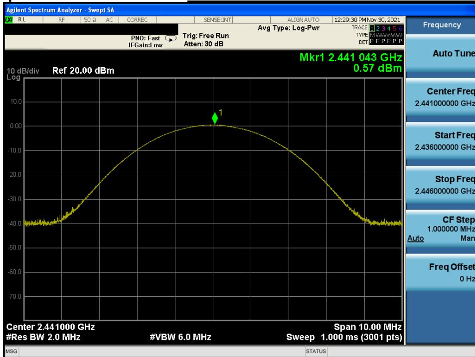
**Peak Output Power****Highest Channel & Modulation : 8DPSK**
