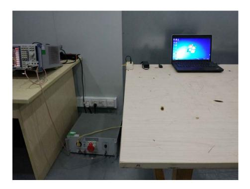
Radiation Emission Test Setup (Below 30MHz)
