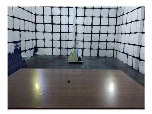
Radiation Emission Test Setup (Above 1GHz)
