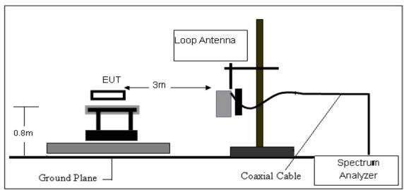
2. Radiated Emission Test-Up Frequency 30MHz~1GHz
