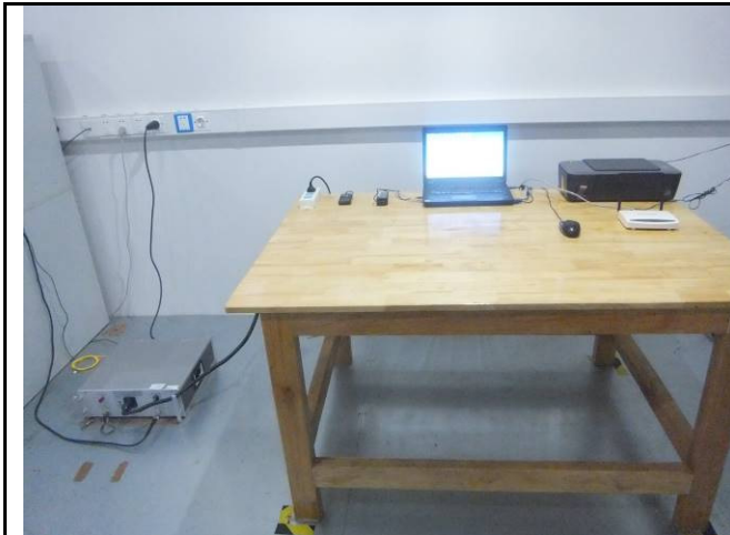
Conducted Emissions Test Setup – Front View
