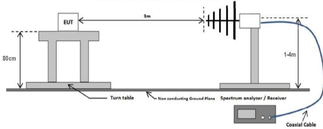
**Radiated emissions test setup above 1 GHz**
