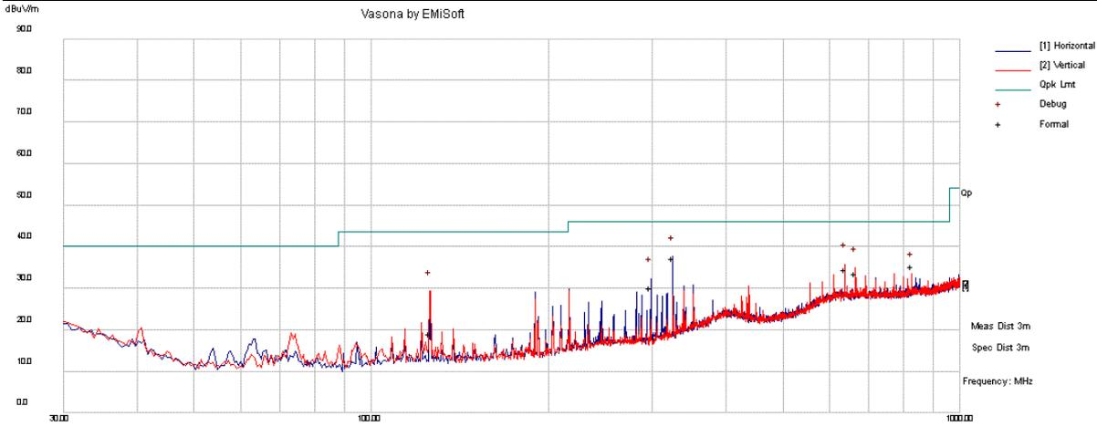
Radiated Emissions Template: FCC Class B (3m) 30MHz-1GHz
