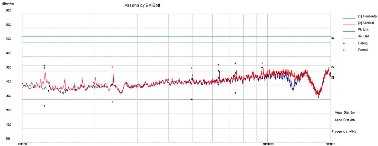
Radiated Emissions Template: FCC 15.209 (3m) 1-18GHz
