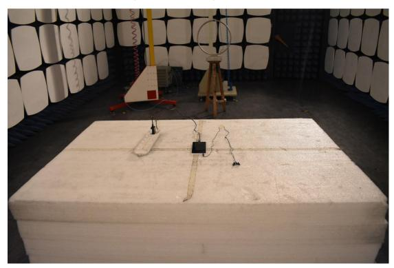
3. Radiated emission (9KHz-30MHz)
