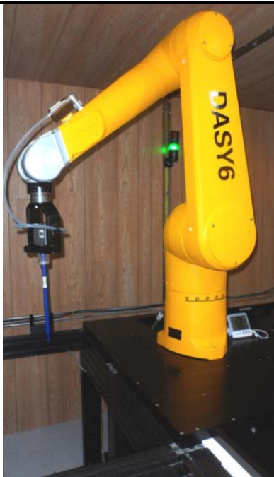
DASY 6 SAR System with SAM Phantom
