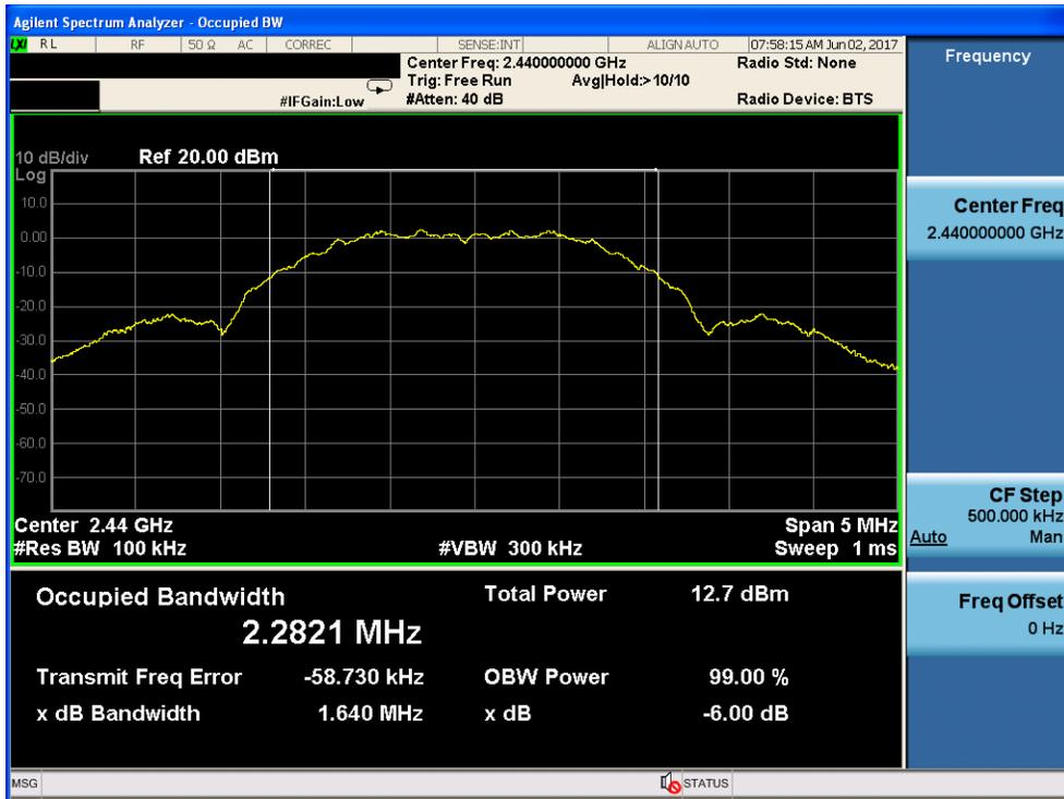
6dB Bandwidth plot on channel 16
