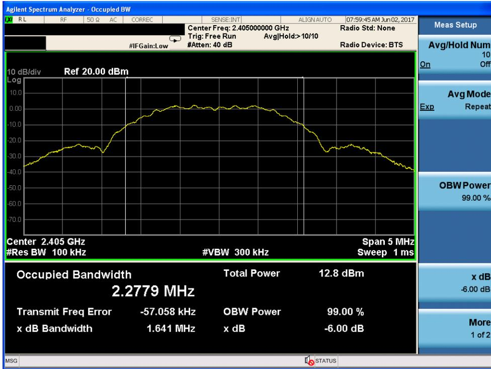
6dB Bandwidth plot on channel 8 1Mbps
