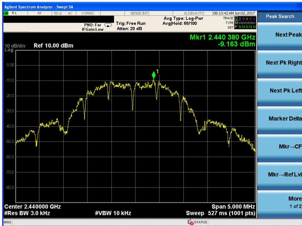
Power spectral density plot on channel 16
