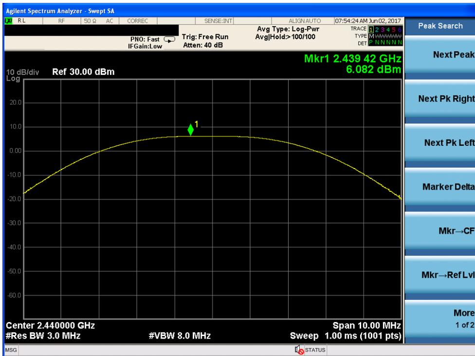
Peak output Power plot on channel 16
