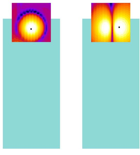
Axial Radial (Transverse) Figure 8-1 T-Coil Scan Overlay Magnetic Field Distributions
