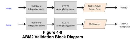
The power summed output results for a known input were compared to the multi-meter results to verify any deviation in the post-processing implemented with the power-sum.
