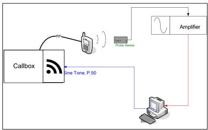
Figure 4-2 T-Coil Test Setup
