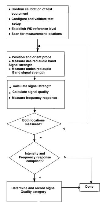
Figure 4-14 C63.19 T-Coil Signal Test Process
