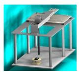
Figure 4-3 RF Near-Field Scanner
