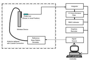
Figure 4-13 **Audio Magnetic Field Test Setup**
