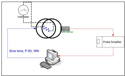
Figure 4-1 Validation Setup with Helmholtz Coil
