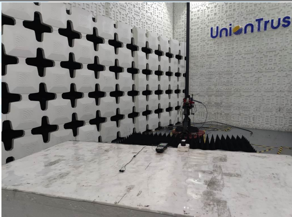
Radiated emission Test Setup-2 (Above 1 GHz) - Test Mode 1&4
