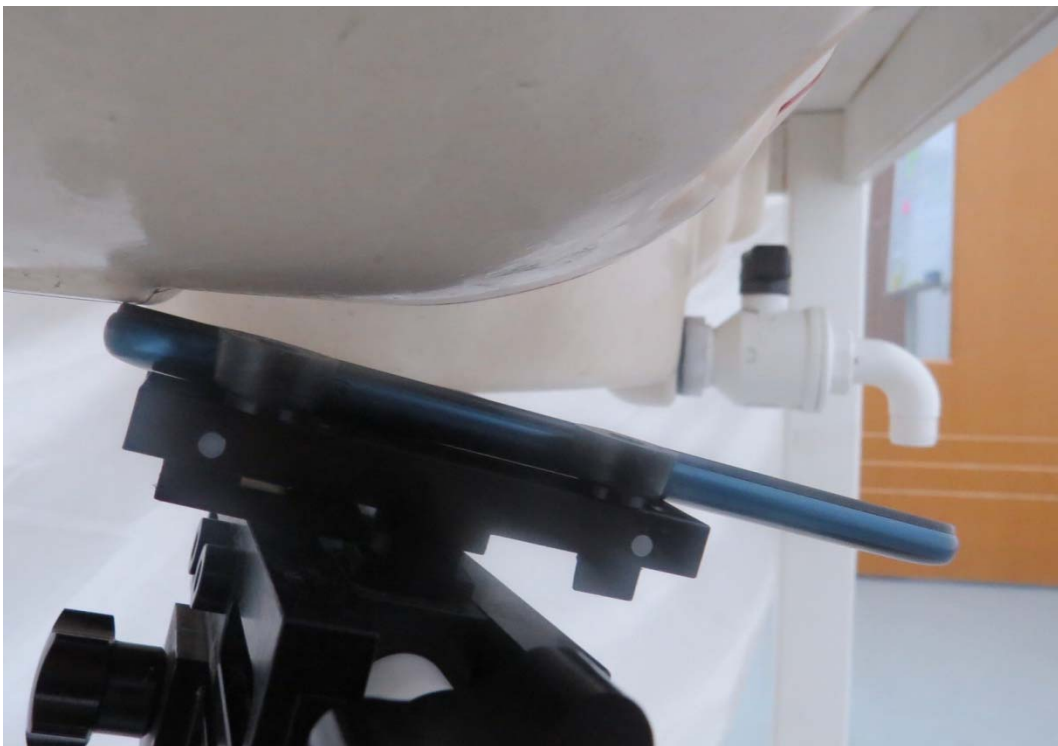
Picture 4: Right Hand Tilt 15 Degree Position
