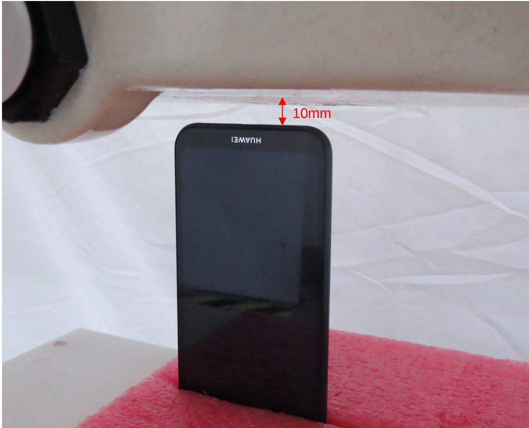
Picture 13: Bottom Edge, the distance from handset to the bottom of the Phantom is 10mm
