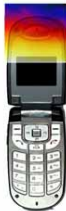
Figure 28 Sample H-field Scan Overlay
