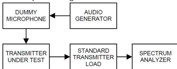
Test setup for Digital:
