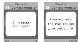
Press menu key to entry registering screen, then push the pair key on the back of baby unit within 10 seconds.
