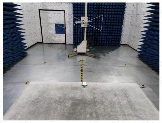
RADIATED EMISSION TEST SETUP ABOVE 1GHz
