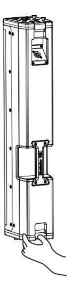
Place the second top on the first upside down, then align the blocking systems and apply pressure to engage. If the assembly is correct, the safety levers move outwards (released position) with a "click".
