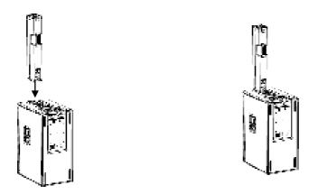
Push inwards the safety levers to arm the blocking systems of the two tops as shown.
