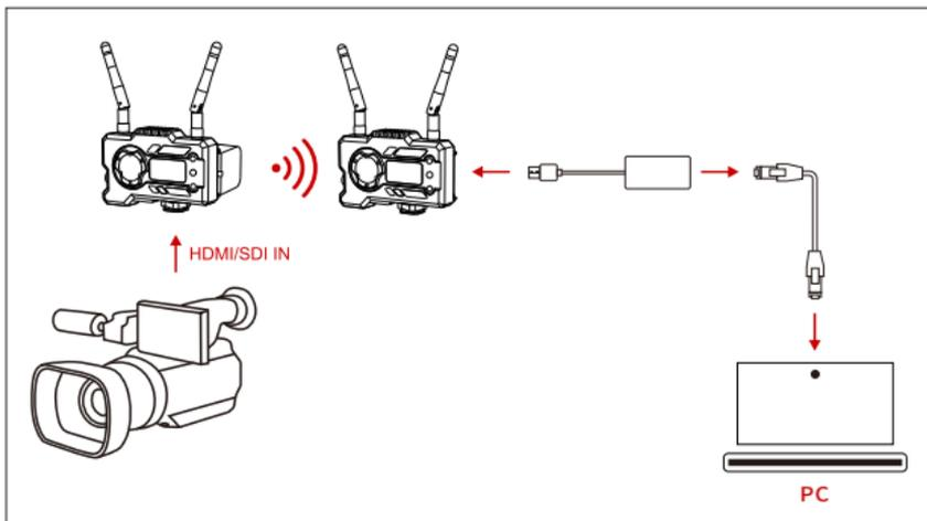
1. Confirm there is video format display on both transmitter and receiver. Use the Type-C to Lan Connector to connect the laptop and RX.
