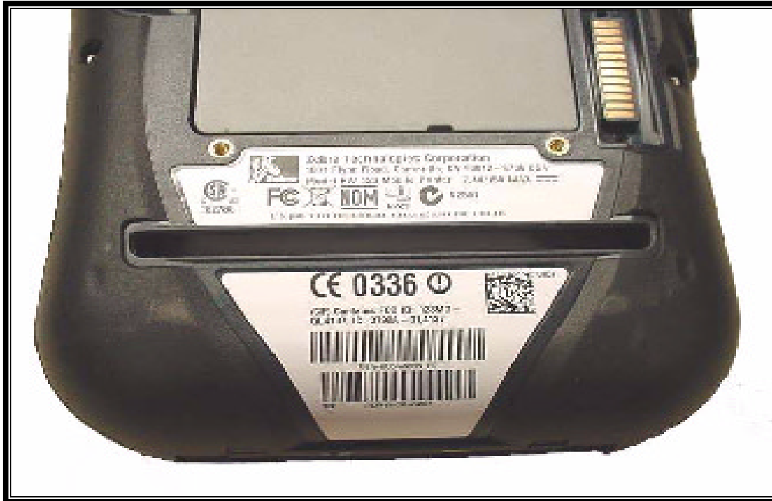
PHOTOGRAPH 4: "CONTAINS FCC ID..." LABEL LOCATION ON PRINTER
