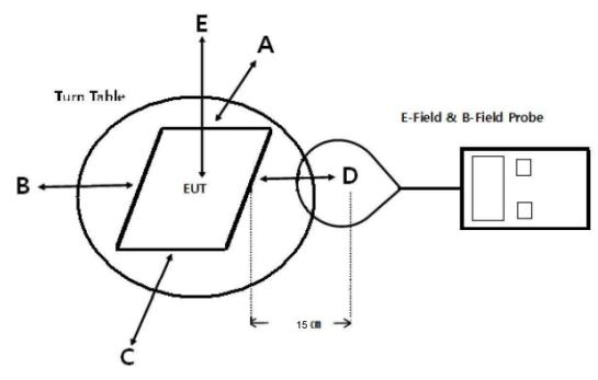
Note: Measurements should be made from all sides and the top of the primary/client pair, with the 15cm measured from the center of the probe(s) to the edge of the device.
