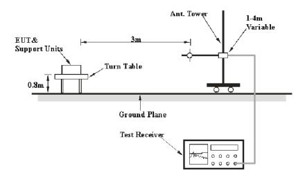
Note: For Below 30MHz test, the Loop Antenna is set above 1.0 meter from ground to the lowest height of loop antenna. Three antenna orientations are set separately (parallel, perpendicular, and ground-parallel) unless the margin is greater than 20 dB
