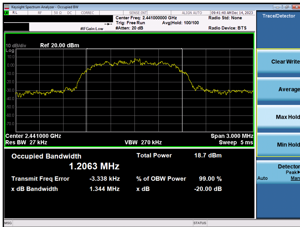
Plot 7-5. 20dB Bandwidth Plot (Bluetooth, 2Mbps – Ch. 39)
