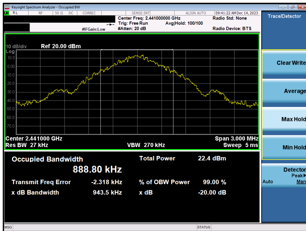
Plot 7-2. 20dB Bandwidth Plot (Bluetooth, 1Mbps – Ch. 39)
