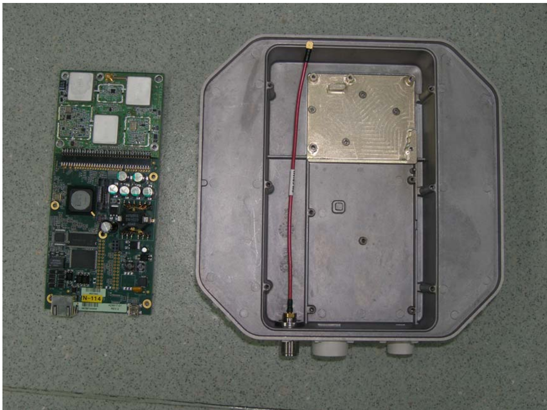
Photo7. CPE with PCB removed , component side
