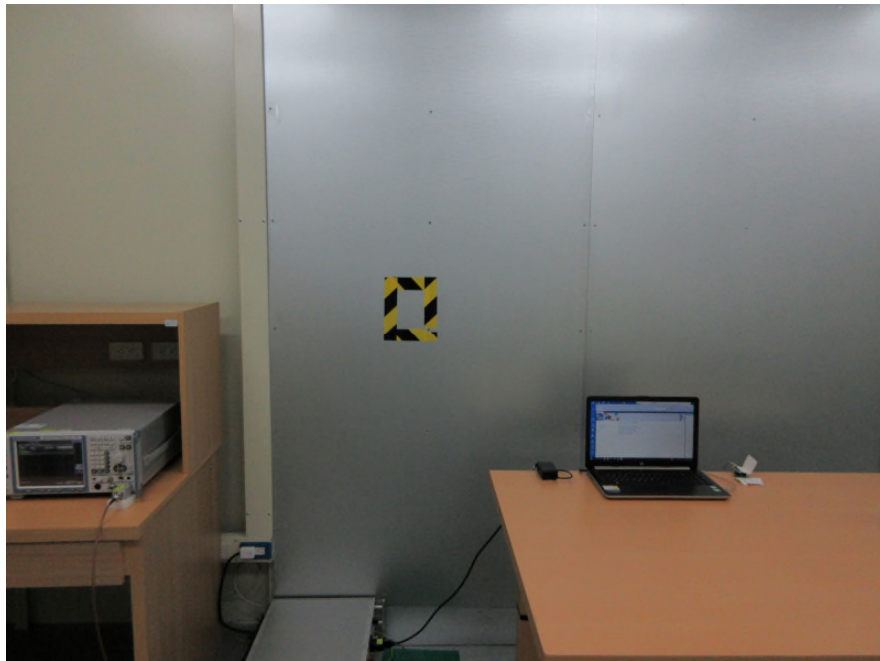
Photograph 6: Set-up for AC Mains Emissions (Front View)
