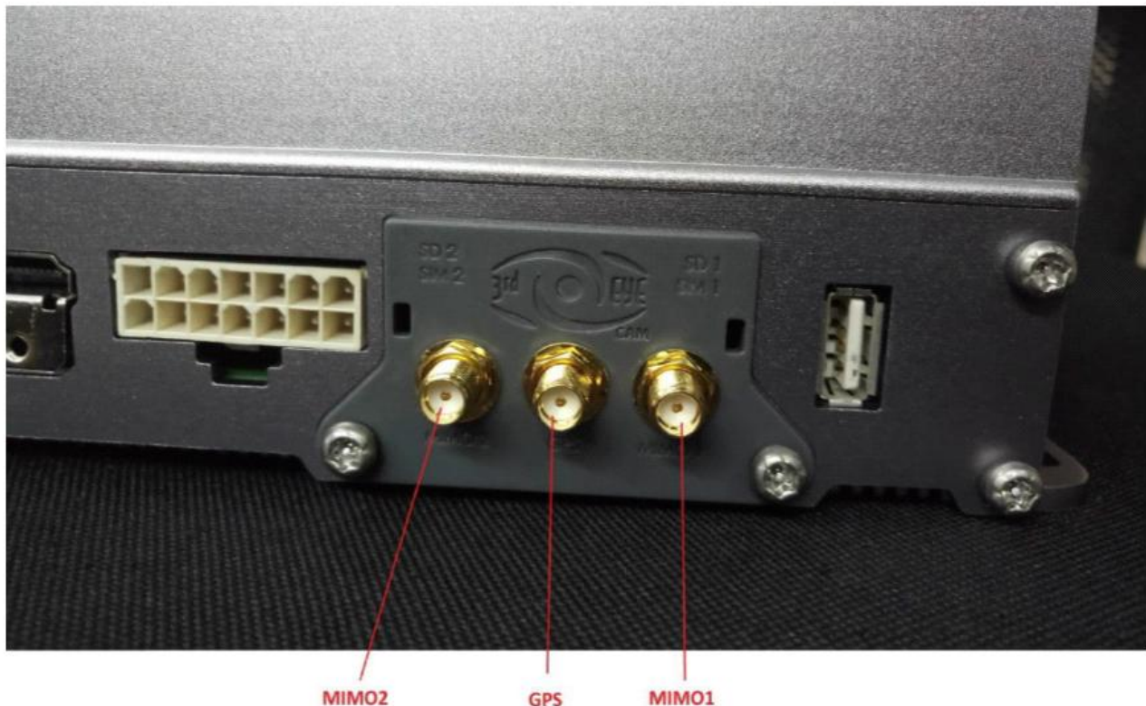
Antenna Connection with packed unit inside mechanical enclosure
