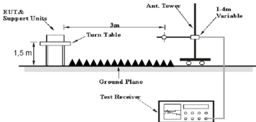
The radiated emission Below 1GHz tests were performed in the 10 meters chambe, above 1GHz tests were performed in the 3 meters chamber A, using the setup accordance with the ANSI C63.10-2013. The specification used was the FCC 15.209, and FCC 15.247 limits.
