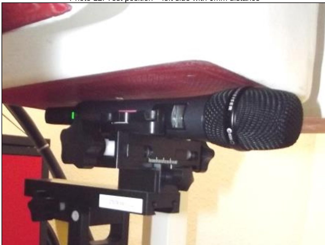
Photo 12: Test position – left side with 0mm distance
