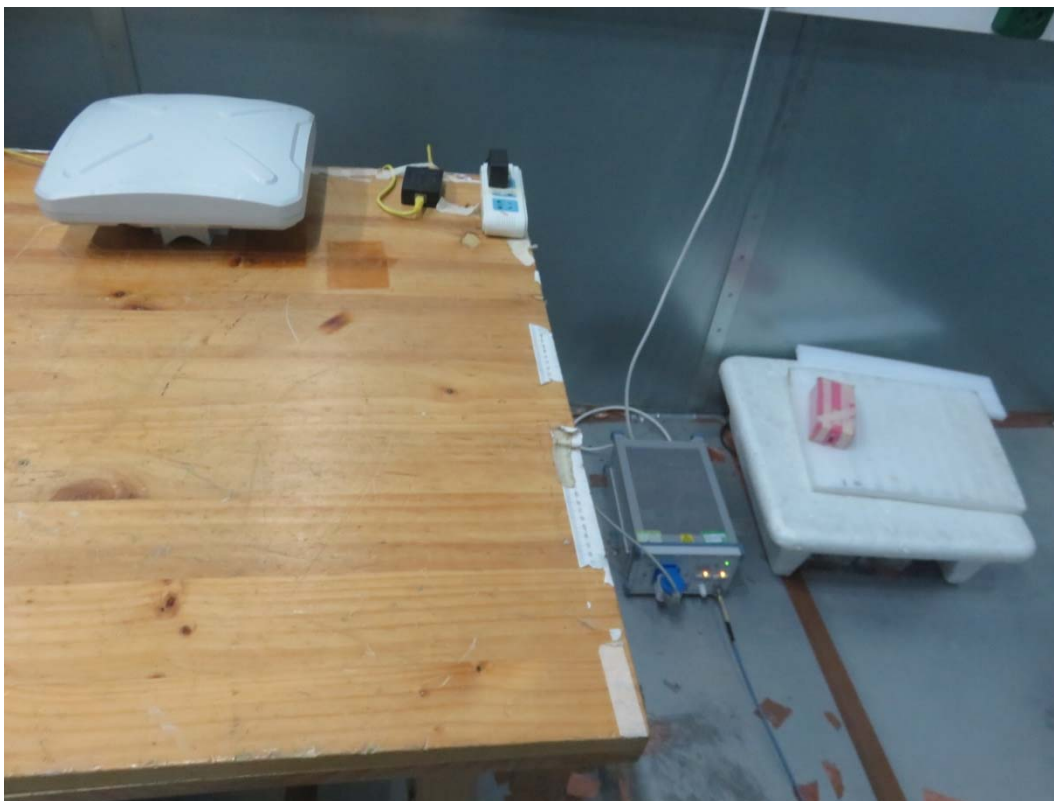
Picture 3 Radiated Emission Test Setup
