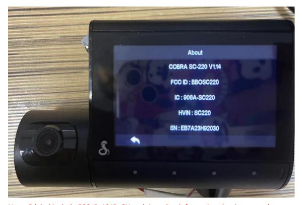
Note: E-label include FCC ID, IC ID, SN and the other information that is not on the device label.
