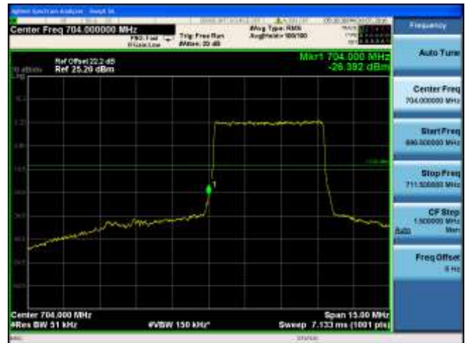
CH23780 (709MHz) QPSK Bandwidth 10MHz 50RB#0
