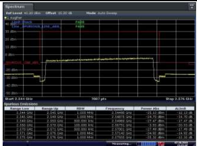
CH21350 (2560MHz) 16QAM Bandwidth 20MHz 100RB#0
