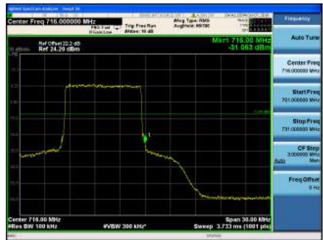
CH23173 (715.3MHz) 16QAM Bandwidth 1.4MHz 6RB#0
