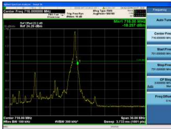
CH23130 (711MHz) 16QAM Bandwidth 10MHz 1RB#49
