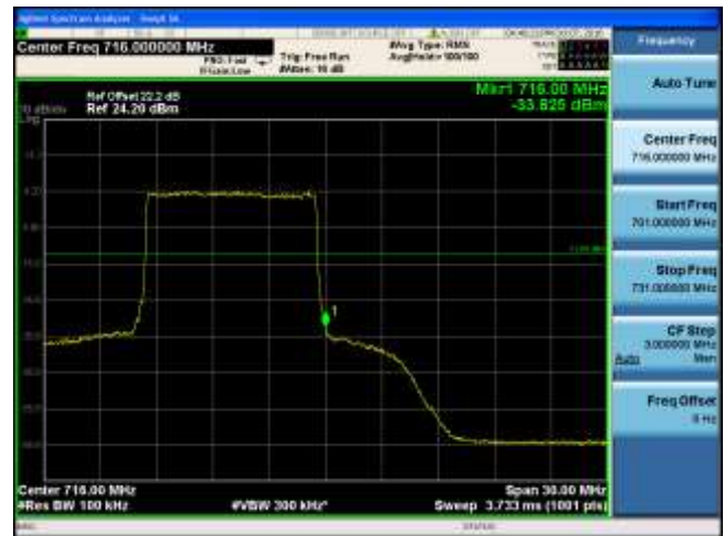
CH23130 (711MHz) 16QAM Bandwidth 10MHz 50RB#0
