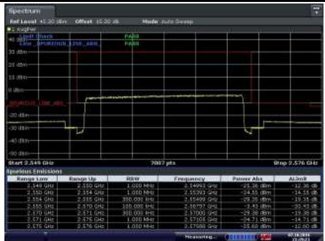
CH21375 (2562.5MHz) 16QAM Bandwidth 15MHz 75RB#0
