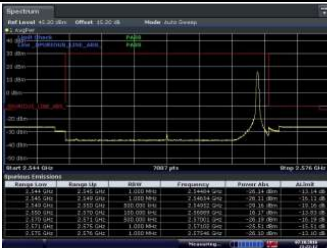
CH21350 (2560MHz) 16QAM Bandwidth 20MHz 1RB#99
