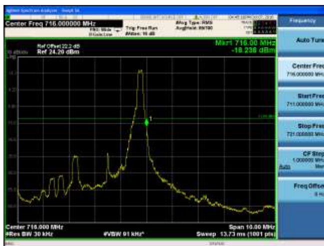
CH23165 (714.5MHz) 16QAM Bandwidth 3MHz 1RB#14
