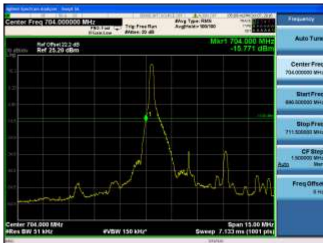
CH23755 (706.5MHz) 16QAM Bandwidth 5MHz 1RB#0
