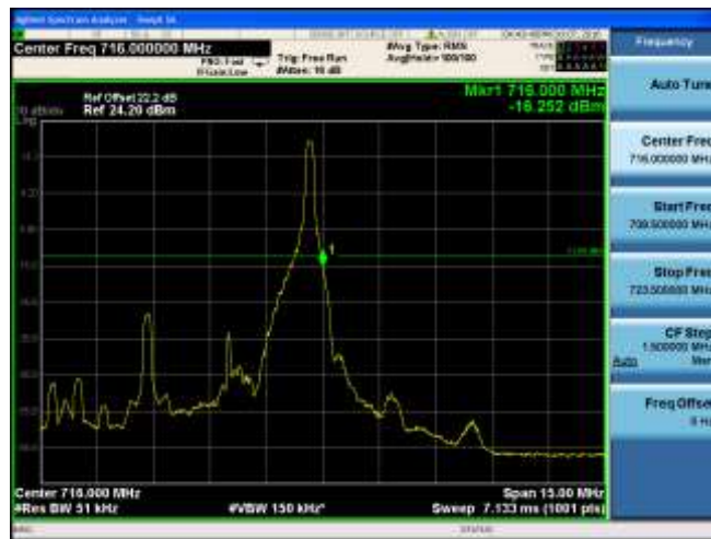
CH23130 (711MHz) 16QAM Bandwidth 10MHz 1RB#49
