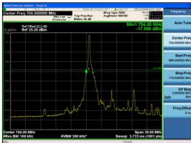
CH23755 (706.5MHz) 16QAM Bandwidth 5MHz 1RB#0
