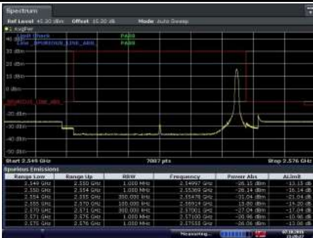
CH21375 (2562.5MHz) 16QAM Bandwidth 15MHz 1RB#74
