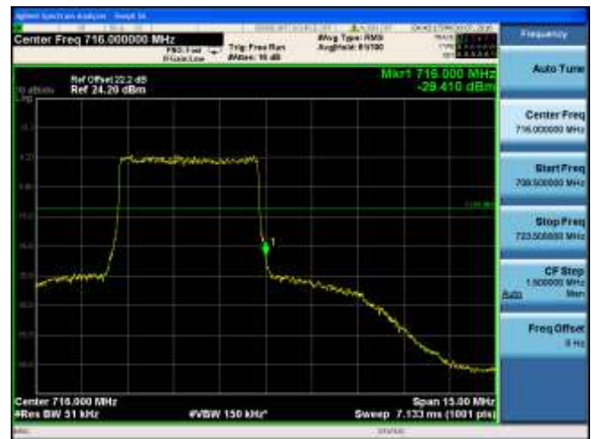
CH23130 (711MHz) 16QAM Bandwidth 10MHz 50RB#0
