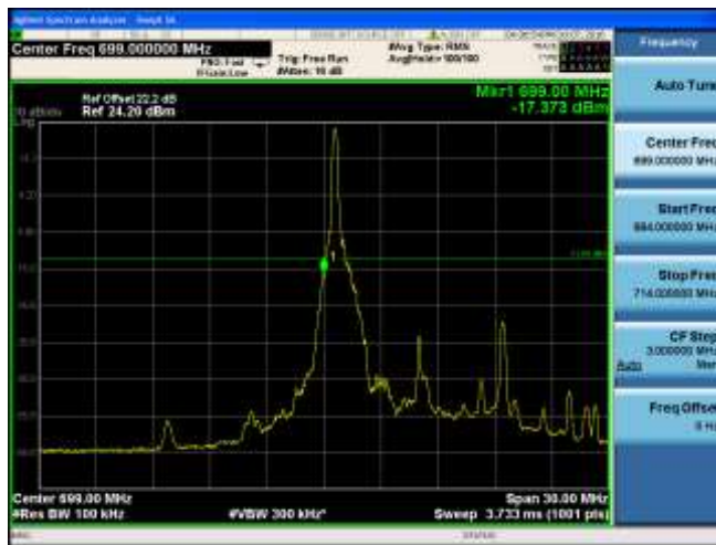
CH20317 (699.7MHz) 16QAM Bandwidth 1.4MHz 1RB#0
