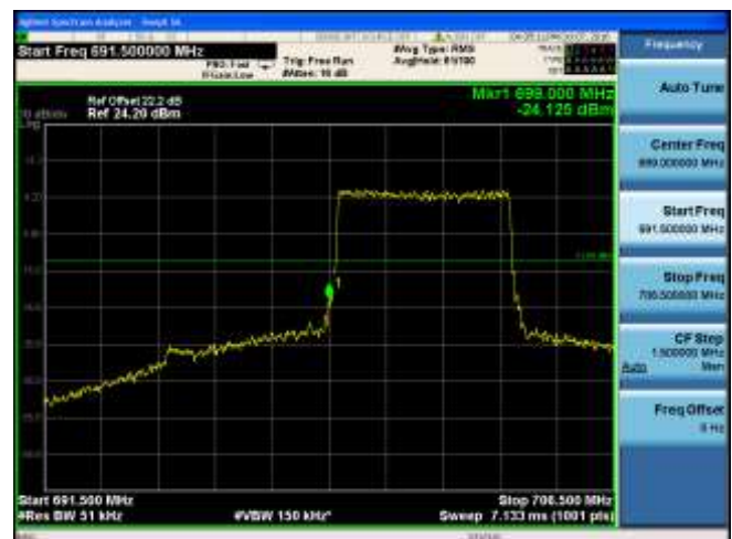
CH23035 (701.5MHz) QPSK Bandwidth 5MHz 25RB#0
