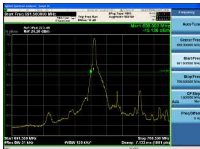
CH23035 (701.5MHz) QPSK Bandwidth 5MHz 1RB#0
