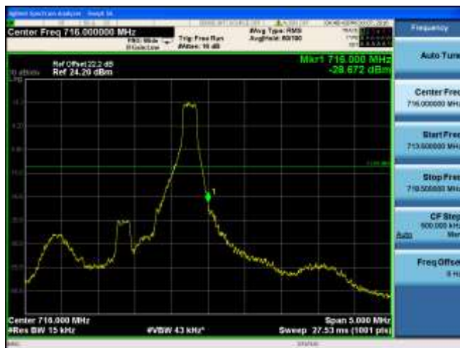
CH23165 (714.5MHz) 16QAM Bandwidth 3MHz 1RB#14
