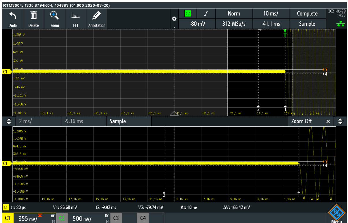
Plot 7.6.9 Transient frequency during power OFF test results at high carrier frequency
