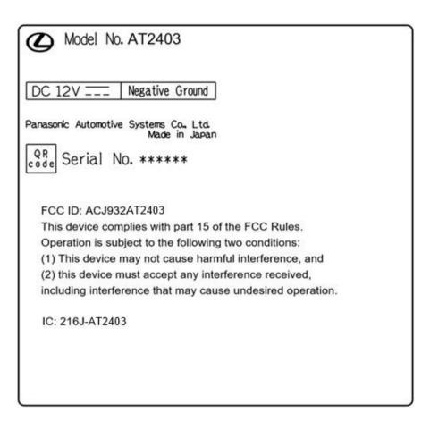
Label display: Printed on paper with ink using a printer and attached to the internal unit Durability of marking: Will withstand expected lifespan without peeling or fading FCC ID character size: 1.5mm
