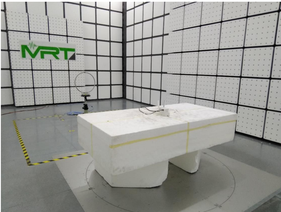
Description: Radiated Emission Test Setup for 9kHz~30MHz
