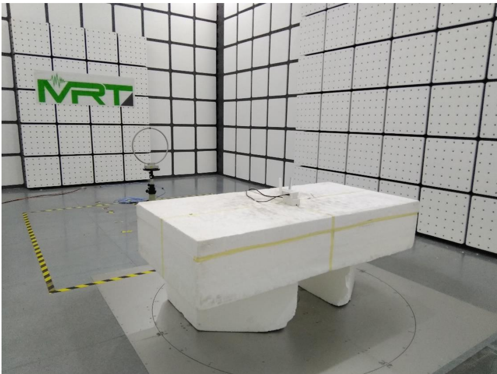
Description: Radiated Emission Test Setup for 9kHz~30MHz
