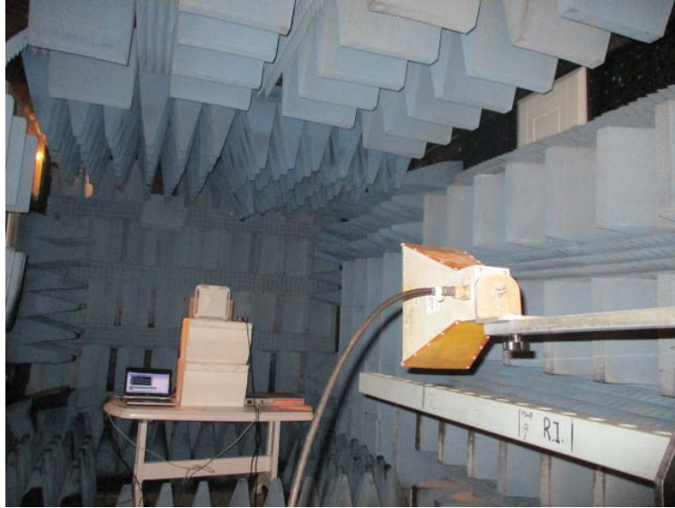
Figure 5. Radiated Emission Test 1-18GHz
