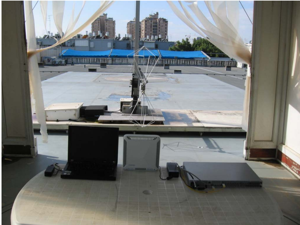
Figure 3. Radiated Emission Test 30 - 200 MHz
