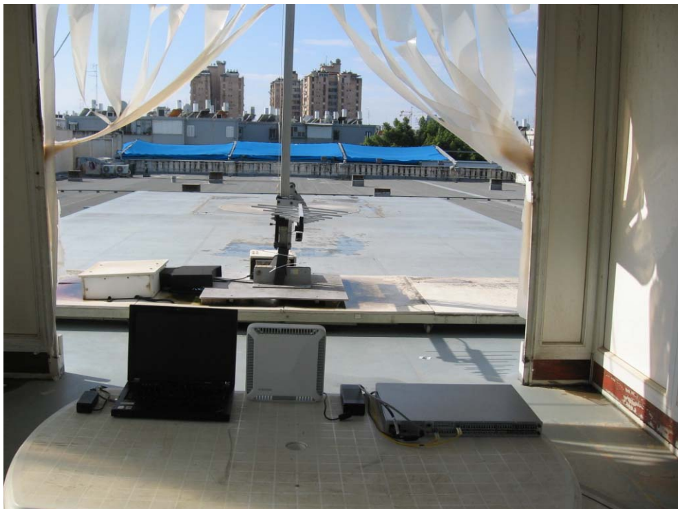
Figure 4. Radiated Emission Test 200 - 1000MHz
