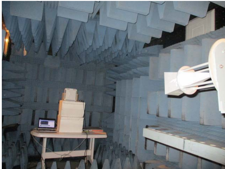
Figure 6. Radiated Emission Test 18-24GHz
