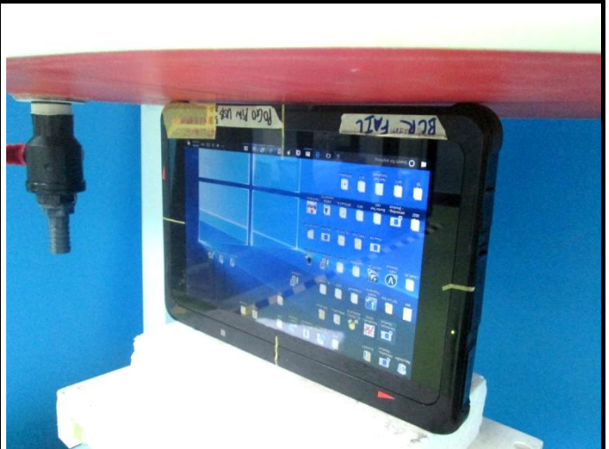
Bottom Side of EUT with 0 cm Gap
