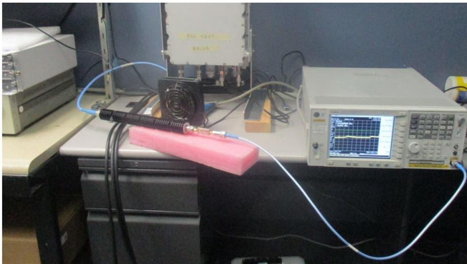
Photograph of 1.2GHz to 8GHz Test Setup
