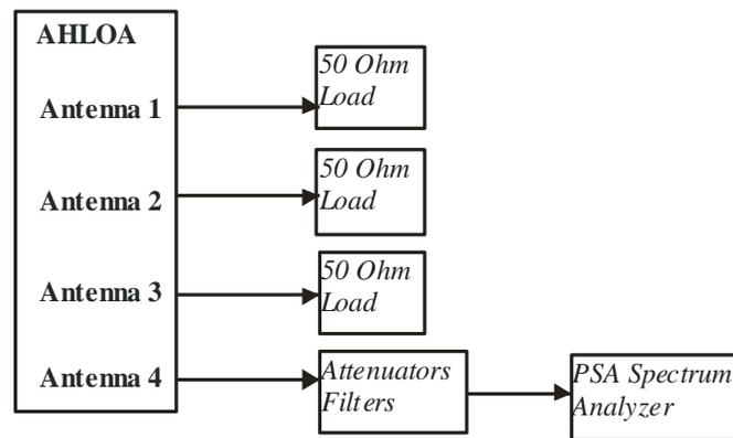
Test Setup Used for AHLOA Conducted RF Measurements
