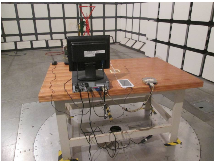
Radiated Emissions – Rear View (Below 1 GHz)
