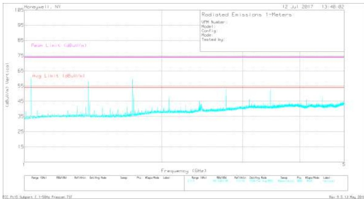
NOTE: Prescans performed in an anechoic chamber, final measurements performed on an OATS
