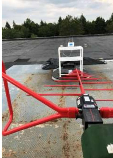
**Test Setup Photos – Radiated Emissions above 1GHz**
