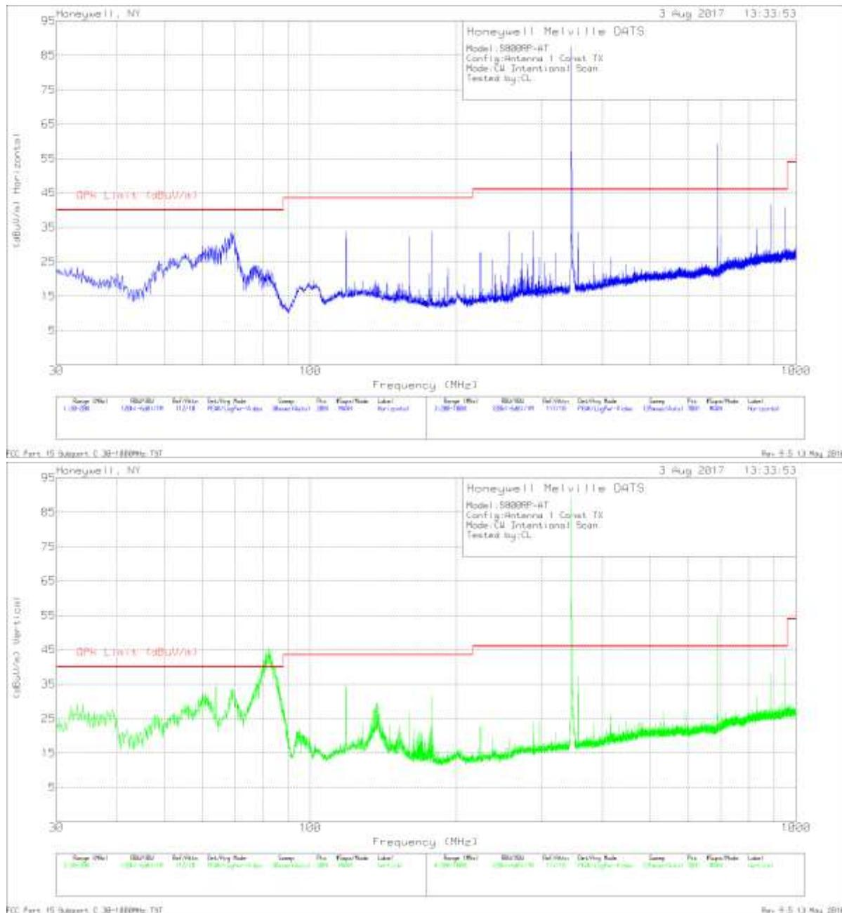
NOTE: Prescans performed in an anechoic chamber, final measurements performed on an OATS
