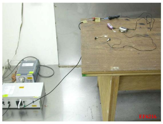
**Photo 2: Conducted Emission Test Set-up**
