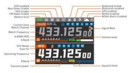
stThe highlighted band is the main channel (i.e., the working band) and the grayed-out band is the sub band (the watch band)  $oldsymbol{\circ}$
