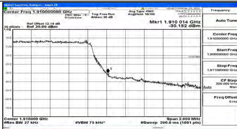
Band Edge Test Graph(s) (Channel Bandwidth: 1.4 MHz)_HCH_QPSK
