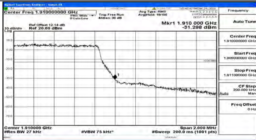
Band Edge Test Graph(s) (Channel Bandwidth: 1.4 MHz)_HCH_16QAM
