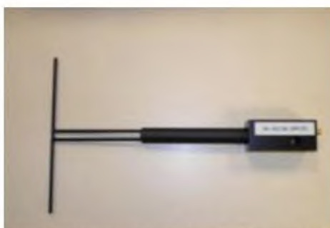
Figure 1 – Satimo COMOSAR Validation Dipole
